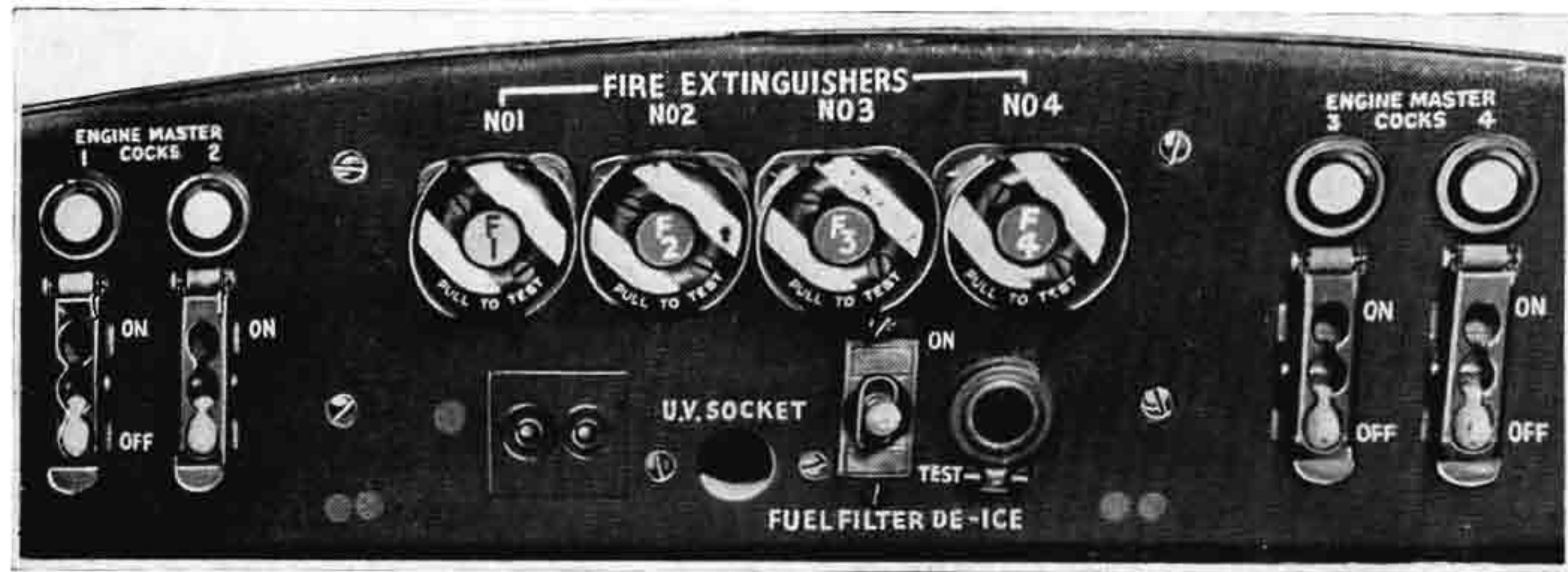
Fig. 29 Engine fire-extinguisher controls
